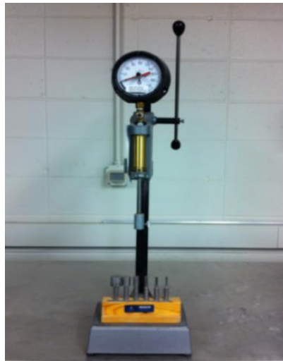
Figure 2. Device for penetration test
